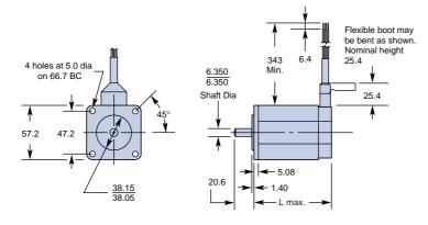
Size 34 Frame, R Series and OEM83 motors, regular construction
