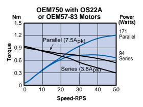
Note: ±10% torque variance due to motor tolerance.
