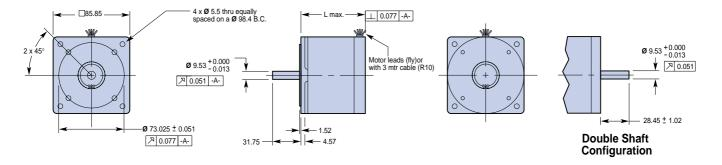
Size 34 Frame, R Series, end bell construction (NPS)
