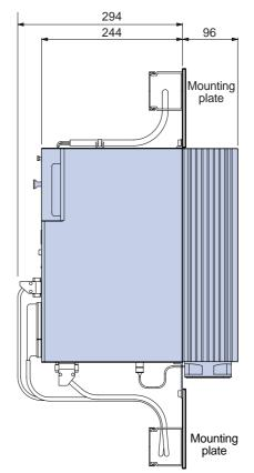
All backplate & bracket fixings accept M6 screws. For through-panel mounting, use brackets type MTS2/01
