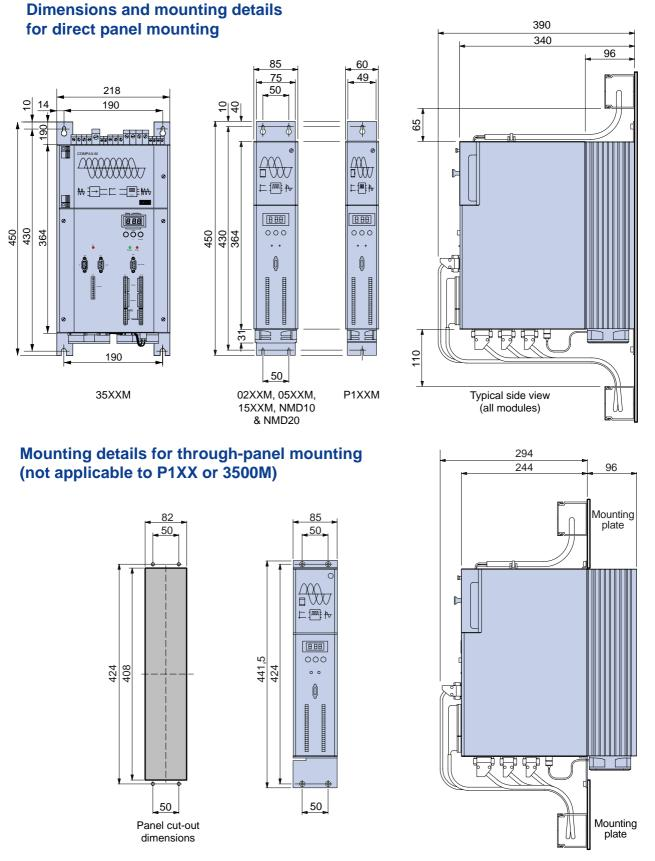
All backplate & bracket fixings accept M6 screws. For through-panel mounting, use brackets type MTS2/01
