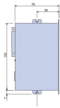
OPTIONAL MOUNTING TABS FOR MINIMUM DEPTH CONFIGURATION
