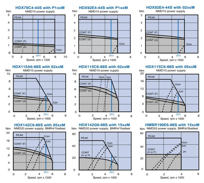
NOTES: 1) Continuous curves: (A) in free air, (F) flange mounted. ΔT = 110°C. Jm = motor inertia.
