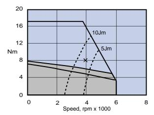
In the example shown, a peak torque of 8Nm and a maximum speed of 4000 rpm are acceptable with a load of 5 times the motor inertia. Note that this information is for general guidance purposes only and will not apply to light duty cycles.
