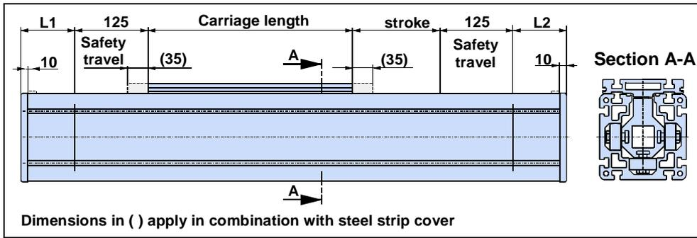
The HLE is also available as a non-driven, idler unit. In this case it acts as a guide only. The profile cross-section and carriage dimensions correspond to those for the driven axes. Please take dimensions L1 and L2 from the following table:
