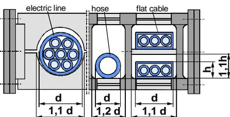
The supply cables must be able to move freely in the cable carrier – they must never be fastened or bundled together. **Separating strips must always** be inserted between flat cables routed in multiple layers.
