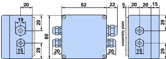
A distribution box with 2.5 m of cable is attached as standard. If a different cable length is required, please specify when ordering.
