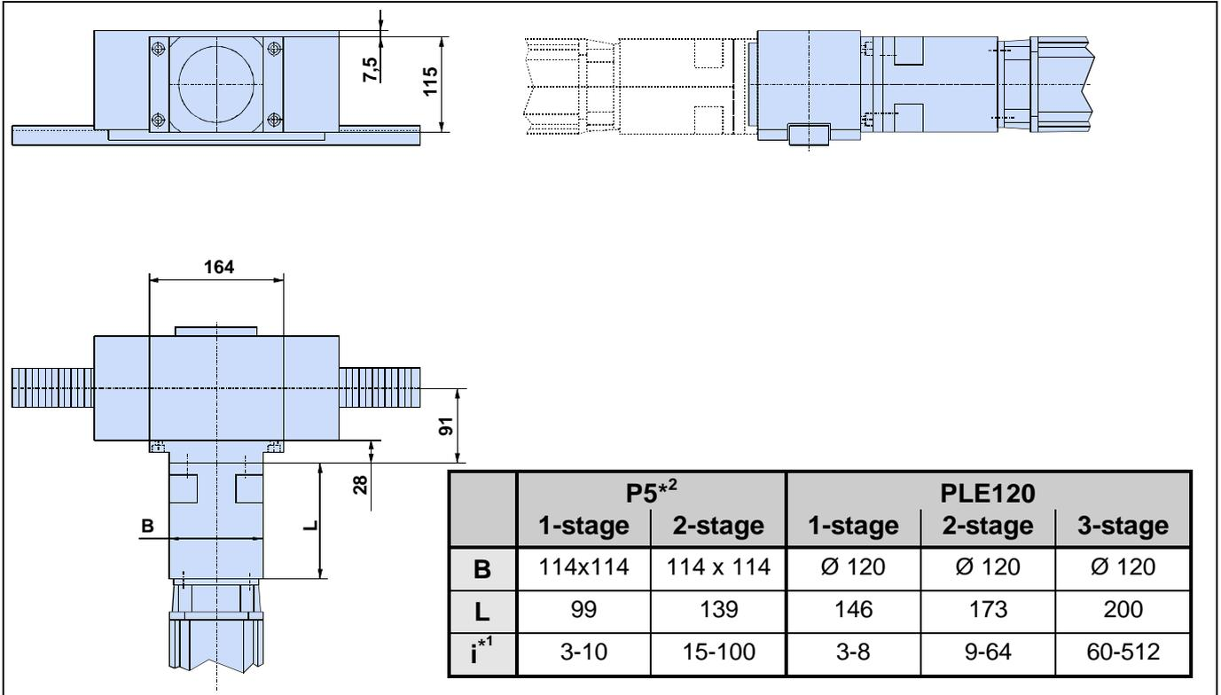
\*1: Ratio range can be supplied; \*2: gearbox P5 compatible with PL115, can be supplied as from August 1999.
