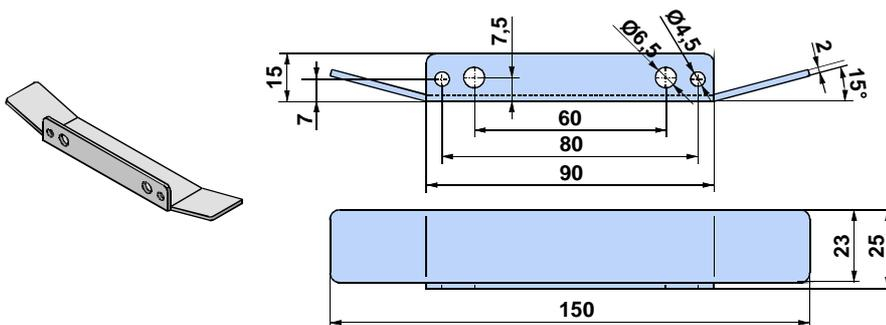
The tripping plate is suitable for all standard load attachment plates. It is mounted at the side of the flange plate using cheese-head screws and square nuts.
