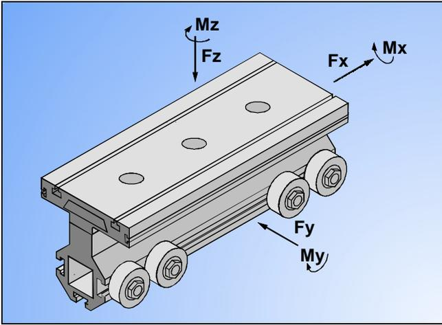
The forces and torques the carriage and the timing belt are capable of transferring are speed-dependent.
