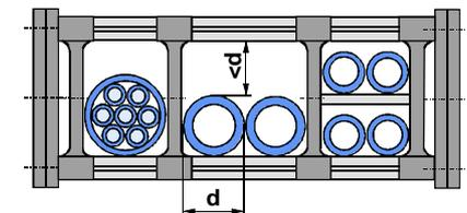
Avoid laying several lines on top of each other and laying lines of different diameters directly next to one another. If multiple layers must be used, separating strips should be inserted between each layer – should such circumstances arise, please contact HAUSER.
