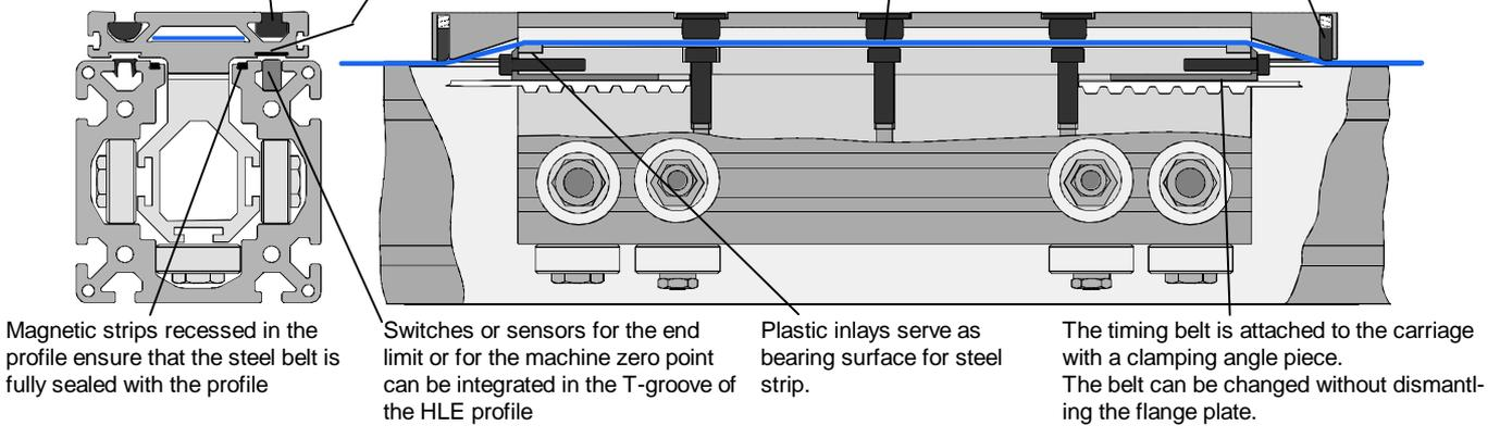
Magnetic strips recessed in the profile ensure that the steel belt is fully sealed with the profile
