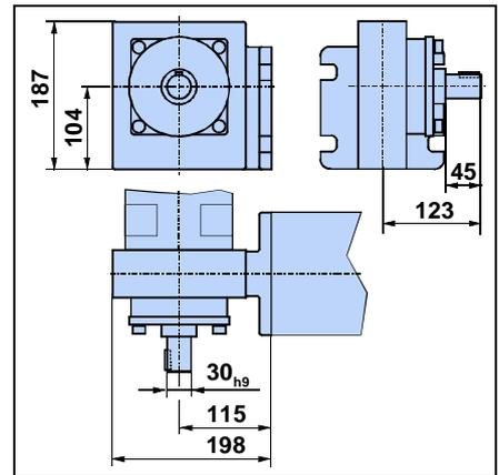
RL: gearbox on right and shaft on left
