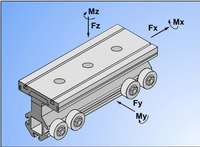
The force and torque ratings of the carriage are speed-dependent. The curves shown in the graphs apply to a standard carriage (S/T).
